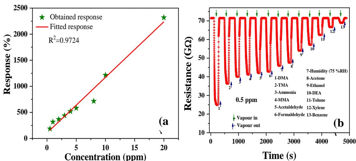
Fig. 4. (a) Linearity plot of  $\alpha$ - $\text{Bi}_2\text{O}_3$  thin film towards dimethylamine vapour towards and (b) Transient plot of  $\alpha$ - $\text{Bi}_2\text{O}_3$  thin film for various reducing vapours.
