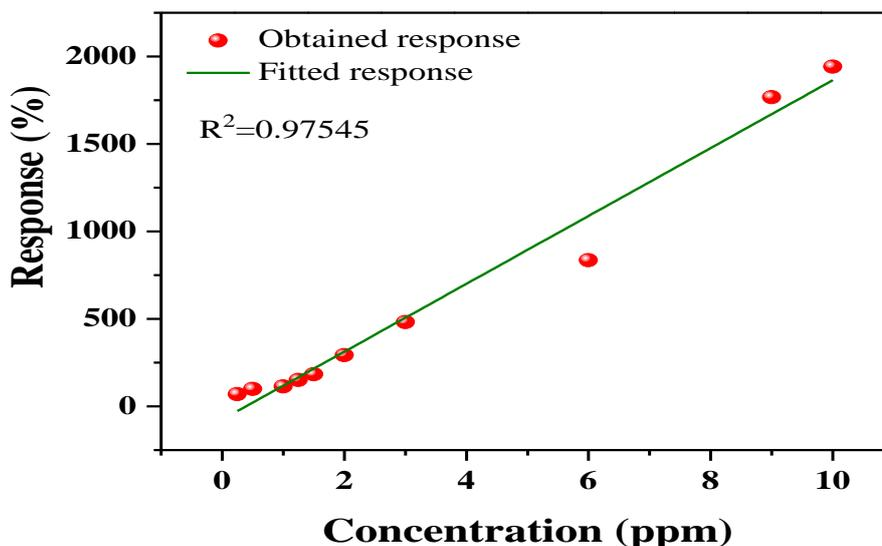
Fig. 3. Acetaldehyde vapour concentration dependent sensing response plot.
