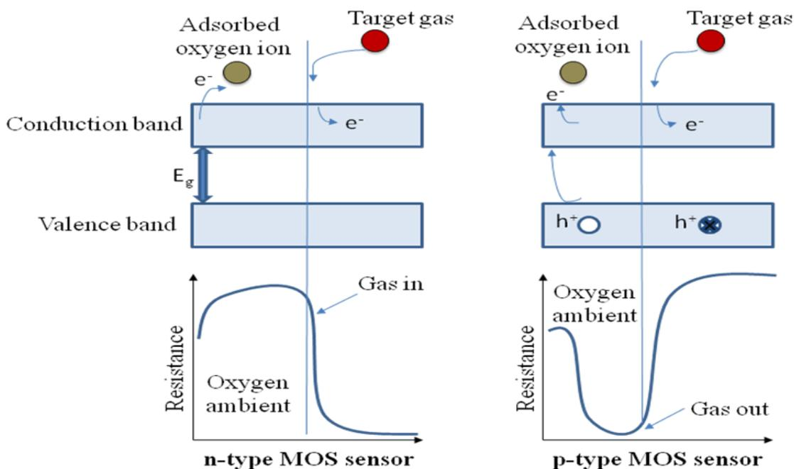
Fig. 1. Electrical Resistance variation based on its semiconducting properties
