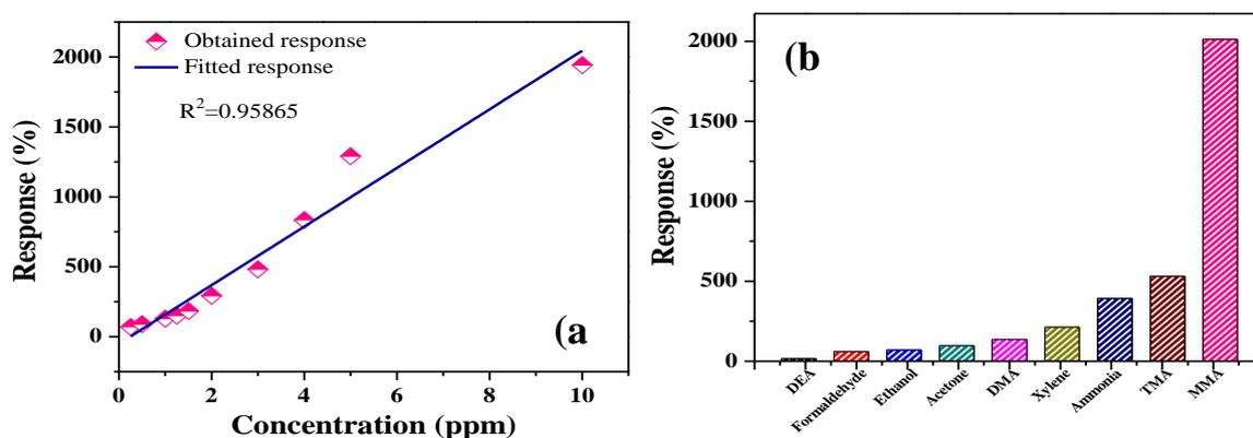
Fig. 5. (a) Monomethylamine concentration dependent sensing response of ZrO<sub>2</sub> thin films. (b) Sensing response of ZrO<sub>2</sub> thin films towards monomethylamine and other reducing vapours at ambient temperature.
